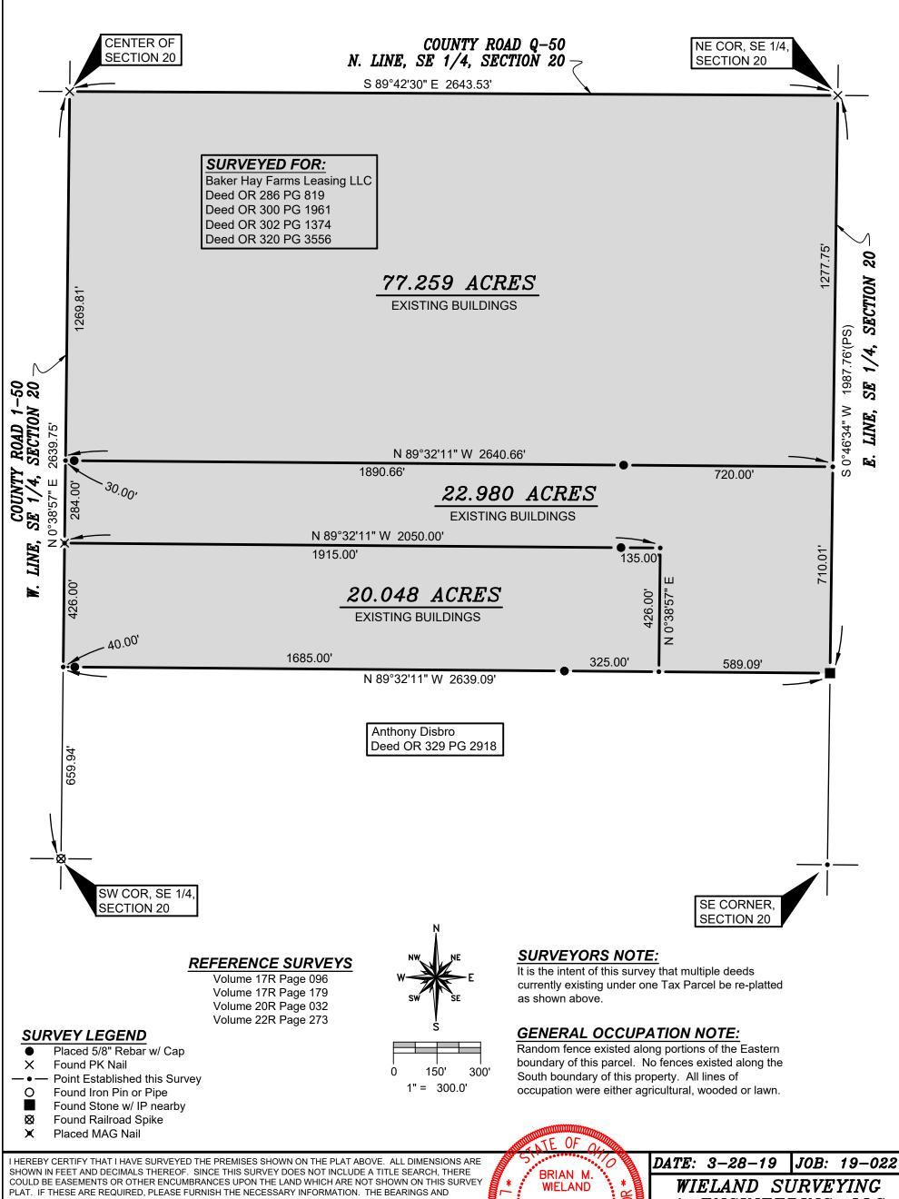
DISTANCES SHOWN ON THE PLAT ABOVE ARE BASED ON STATE PLANE COORDINATES, SPC83, ZONE-OHIO NORTH THIS SURVEY HAS BEEN RECORDED IN VOL.  $\underline{27R}$  PAGE  $\underline{224}$  OF THE WILLIAMS COUNTY SURVEY RECORDS.
